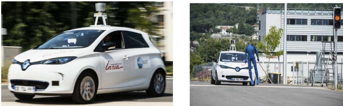
Figure 19: Experimental Platform: Renault Zoe car equipped with Velodyne HDL-64, 4 Ibeo Lux LiDARs, Xsens IMU and cameras, and a crash test dummy crossing the dedicated street for the experiments.
