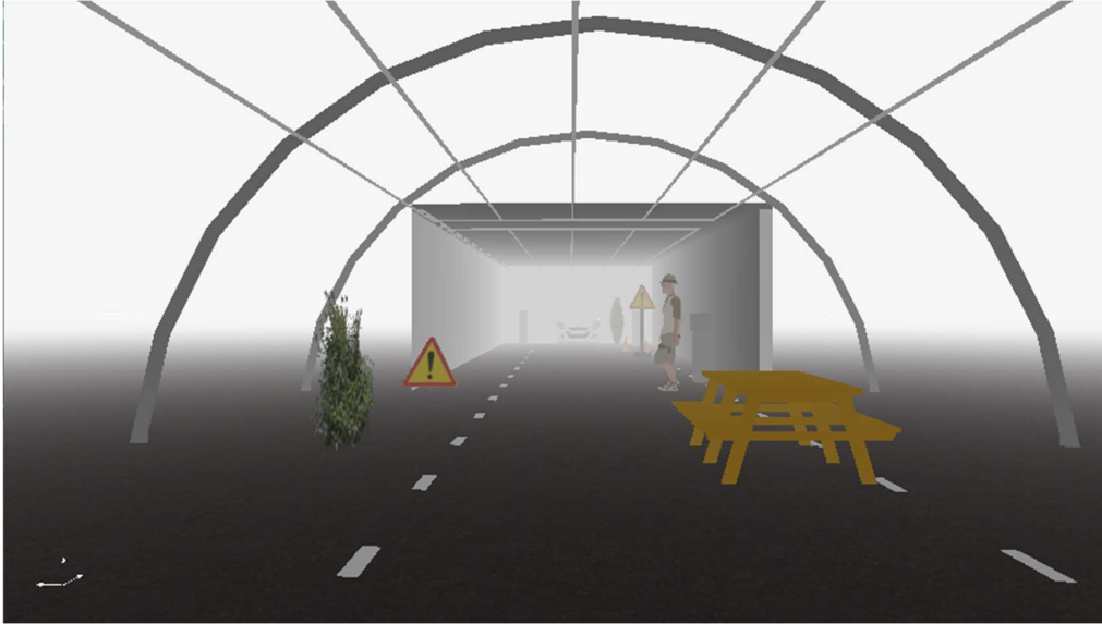
Figure 13: Example of image perceived by the simulated ZED2 camera using 4DV software
