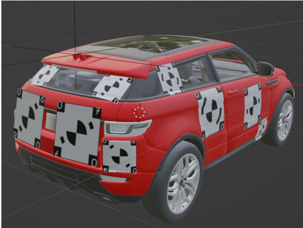
Example of targets implantation on a vehicle
