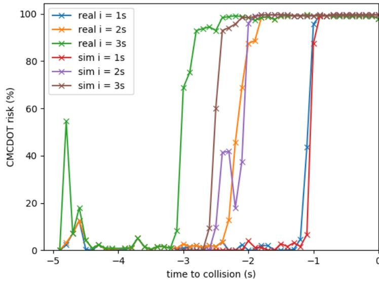
Figure 2: Comparison of real-world and simulated estimations. Curves show CMCDOT risk in  $i$  seconds for real and simulated traces.
