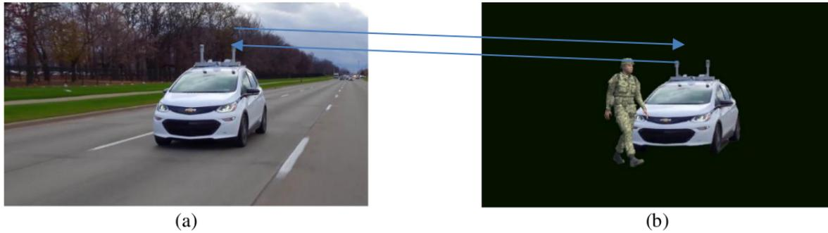
Figure 3: Image from [12]. An illustration of a test conducted with the help of augmented reality. (a) A real vehicle is moving on a real road without any obstacles. (b) A virtual obstacle is added to the vehicle's environment and the sensor information used for testing is a combination of real and virtual objects.
