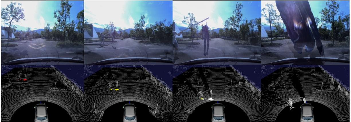
Figure 1: Illustration of one of the experiments performed with INRIA’s autonomous car. The scenario reproduces the car colliding with a pedestrian (mannequin) crossing the street. Top: camera view from the car. Bottom: the environment as seen by the LiDAR and the CMCDOT collision risk grid. The sequence from left to right represents different time stamps. Colors represent probability of collision in 3s (red), 2s (yellow) and 1s (white).
