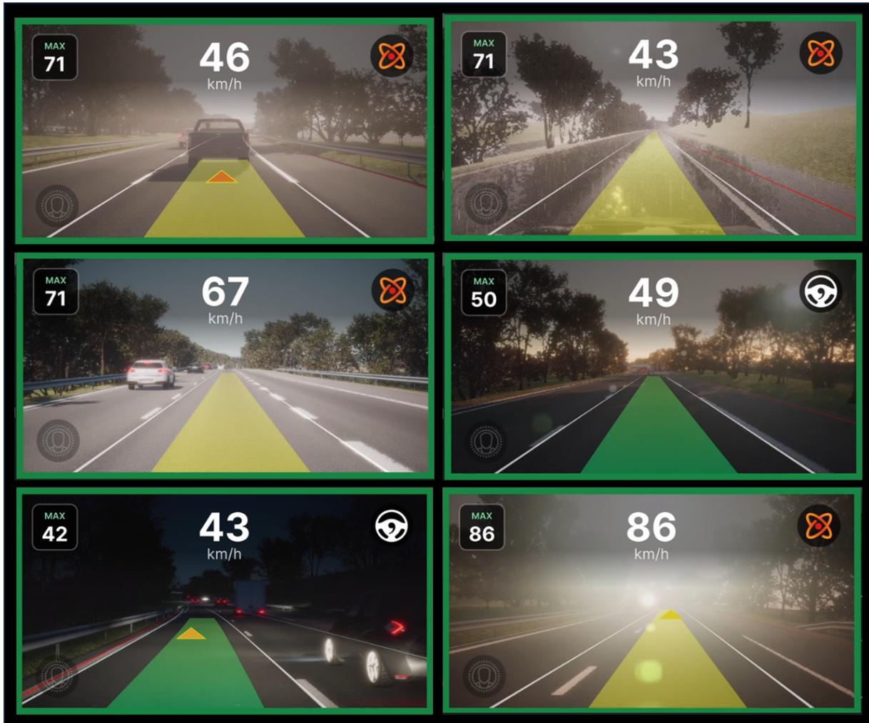
Figure 146: Tests of Openpilot in diverse weather and time conditions in SCANeR studio
