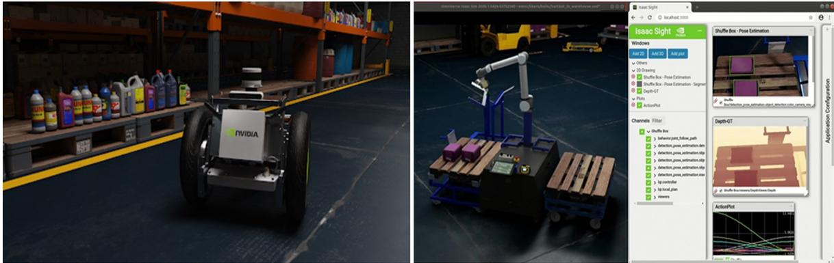
Figure 24: Isaac Sim based on Unreal engine, RTX for photorealism rendering, MDL materials for physically based rendering, and PhysX for dynamic modelling and objects interactions
