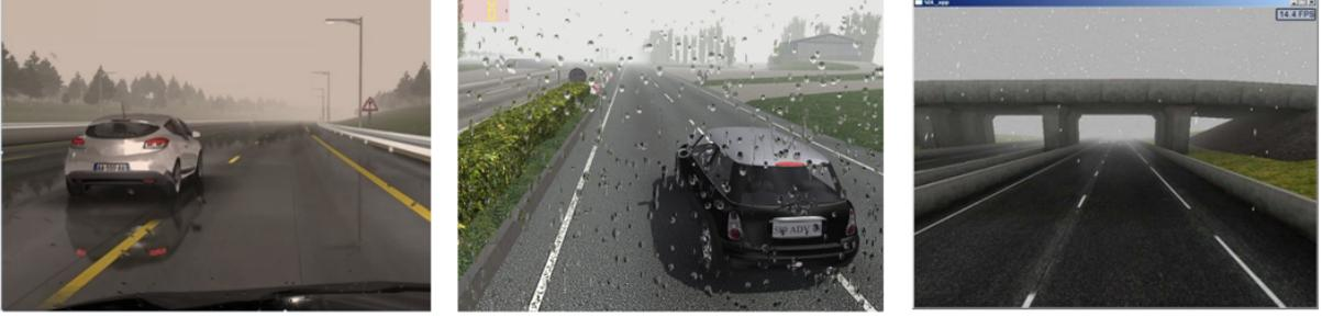
Figure 95: Rain and snow effect in simulated images of ProSivic (specular reflection on wet materials, drops on windscreens and snow on roads) - source UGE.
