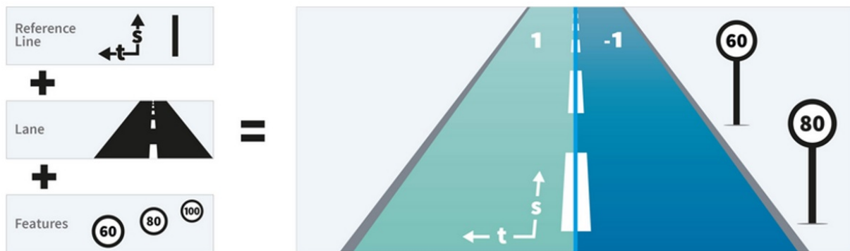
Figure 25: OpenDRIVE road network description
