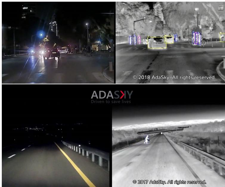
Figure 39: AdaSky's VIPER sensor with a 720p resolution by night
