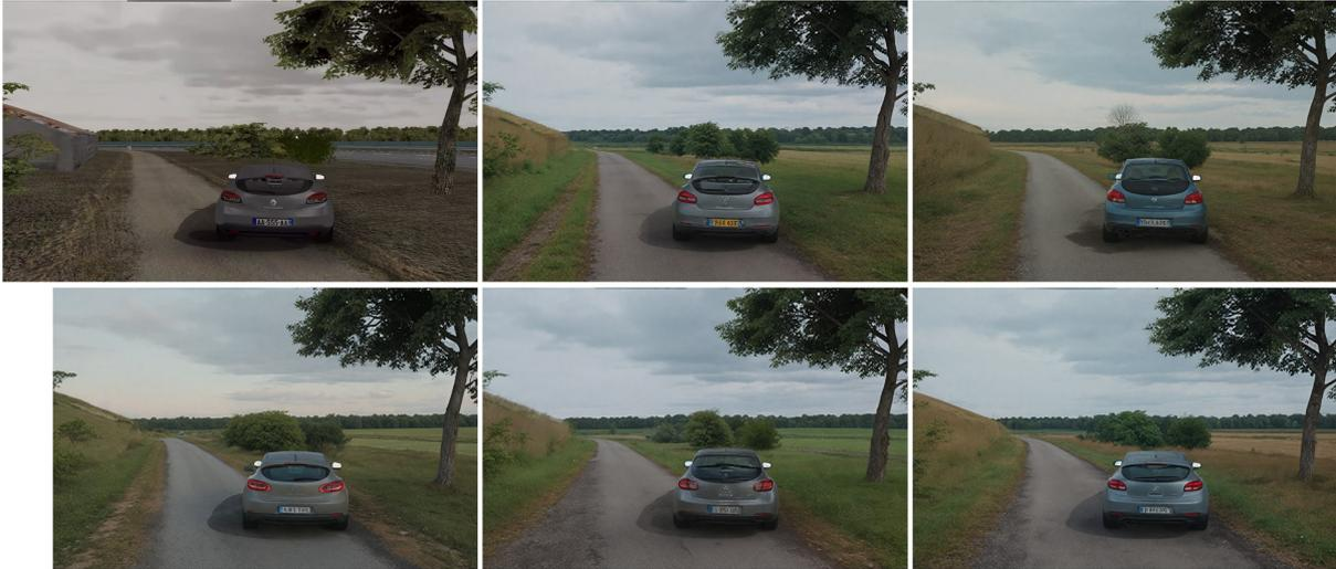
Figure 196: Improvement of the quality of the rendering for a synthetic image generated from Pro-SiVIC on the Transpolis' test tracks. The top left image is the initial image generated from Pro-SiVIC. The other images are generated from AI-based methods with a variation of some parameters (Source: UGE).
