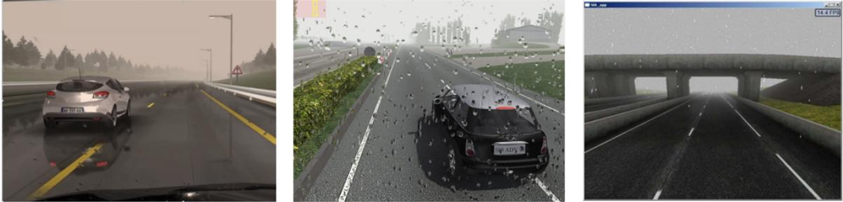
Figure 178: Rain and snow effect in simulated images of Pro-Sivic (specular reflection on wet materials, drops on windcreens and snow on roads) - (source UGE)
