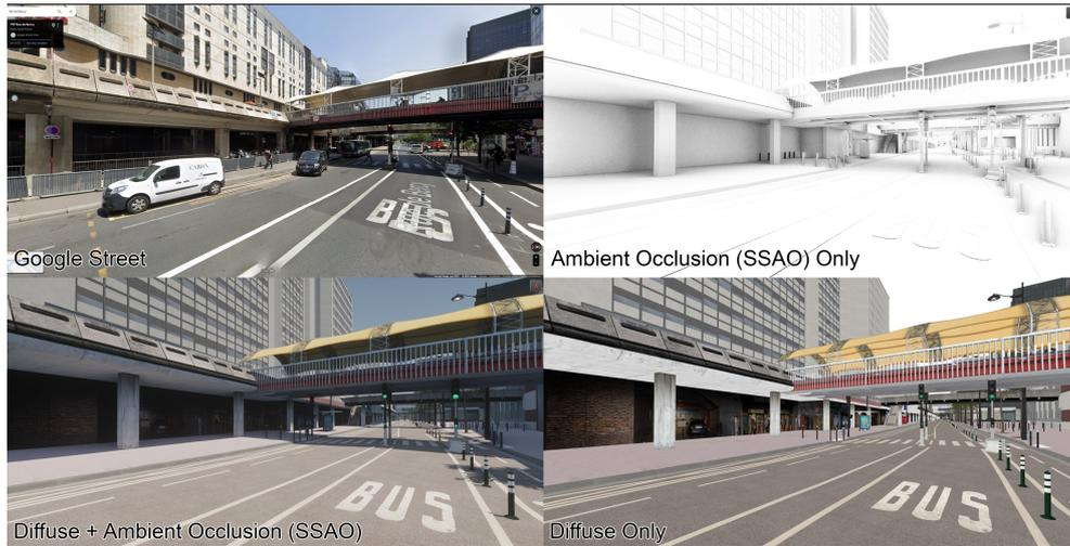
Figure 73: Digital Model and Ambient Occlusion Map, a mandatory rendering mechanism in order to improve significantly the image fidelity (source: UGE and VALEO).
