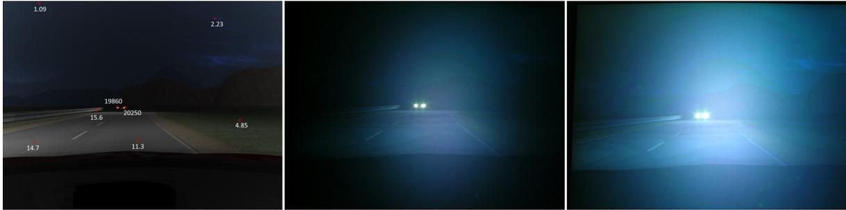
Figure 35: High Dynamic Range (HDR) texture for the light intensity encoding (in Pro-SiVIC). This mechanism is essential in order to generate light blurring and artefact on the camera rendering (source: UGE)
